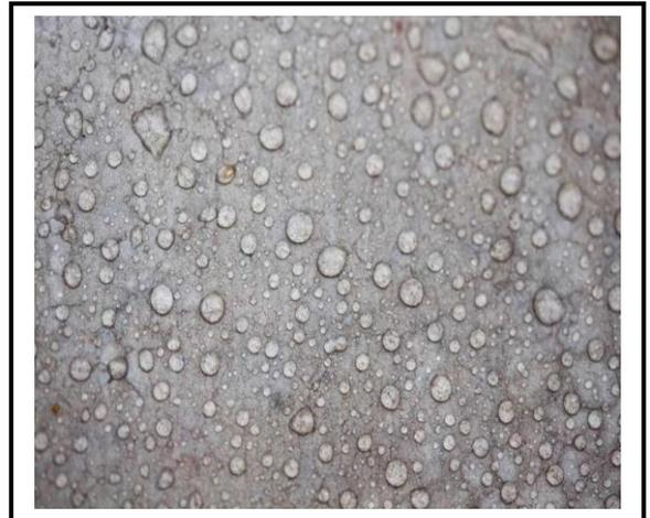
Permanent curing compounds will inhibit the bond of any mortar used for installing ceramic tile and stone because the curing compound has filled all of the pores of the concrete; this means the mortar gets little or no mechanical bond to the concrete.
